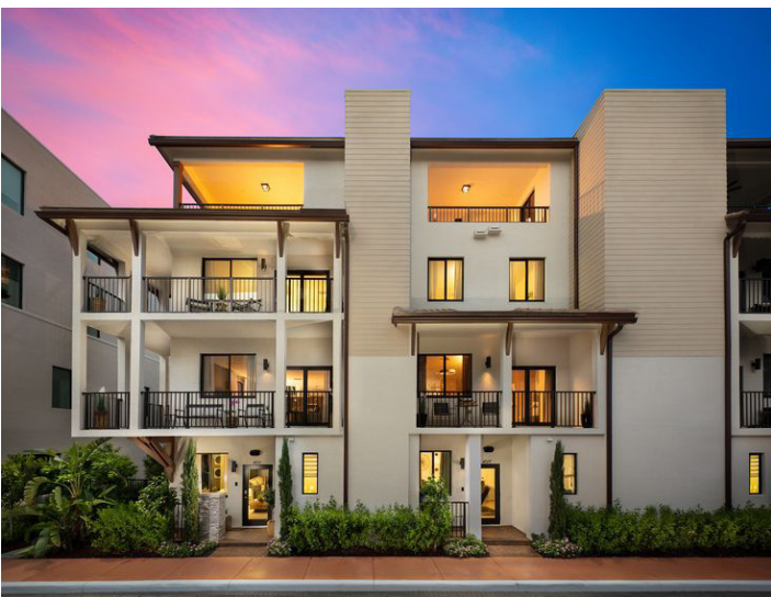
Do - An elevated floor level or setback creates additional privacy for ground floor residential units. Stoops and porches create outdoor open space for ground level units.
